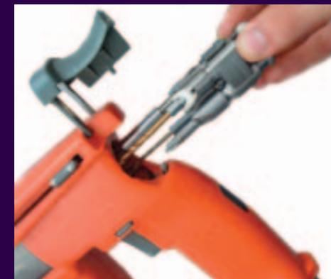
To change damaged or broken tools or just to load a different set of tools, part of the magazine can be ejected through a door in the rear. The cartridge can either be swapped with a second cartridge containing a totally new set of tool bits or individual tools can be unclipped and replaced. The cartridge is then replaced and the door shut.
